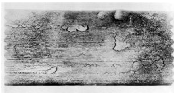
Figure 3-51. Scabs on the Surface of a Rolled Bloom
