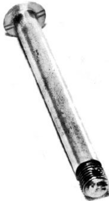
Figure 3-74. Non-Relevant Indications under the Head Created by Slot in Bolt
