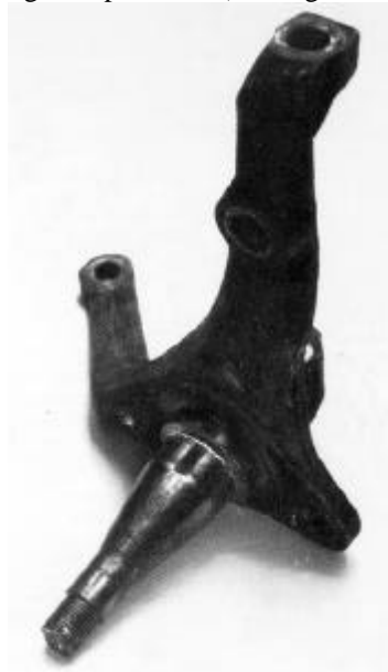
Figure 3-67. Magnetic Particle Indication of a Typical Fatigue Crack.
