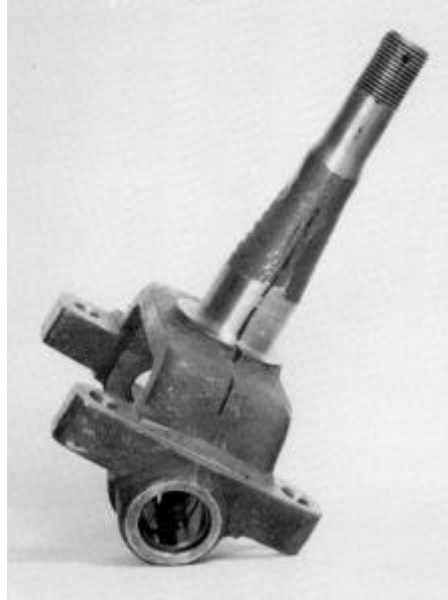
Figure 3-61. Magnetic Particle Indication of Flash Line Tear in a Partially Machined Automotive Spindle Forging.
