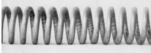
Figure 3-66. Magnetic Particle Indications of Plating Cracks.
