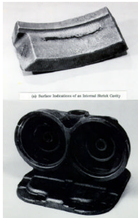
Figure 3-62. Magnetic Particle Indications of Defects in Castings.
