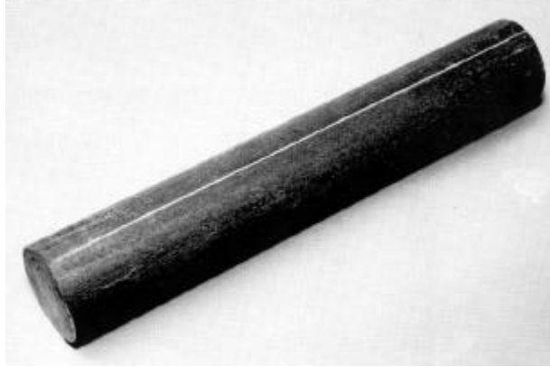
Figure 3-53. Magnetic Particle Indication of a Seam on a Bar.
