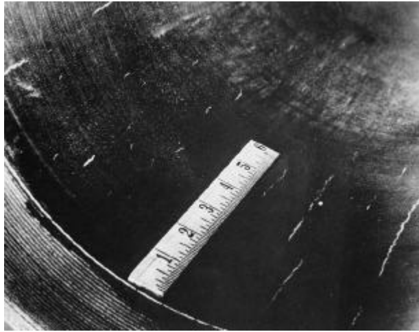
Figure 3-57. Magnetic Particle Indications of Flakes in a Bore of a Large Hollow Shaft.
