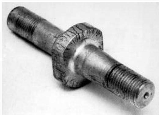
Figure 3-58. Magnetic Particle Indications of Forging Cracks or Bursts in an Upset Section Severe Case.
