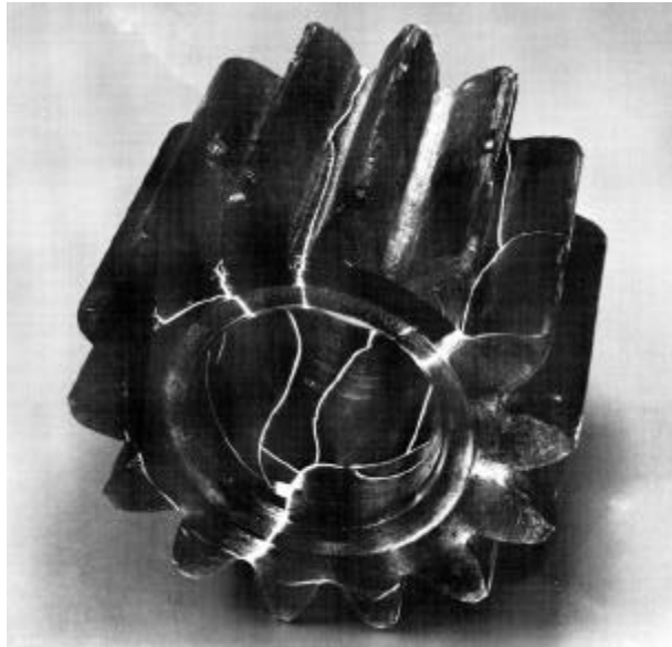
Figure 3-44. Typical Magnetic Particle Indications of Cracks
