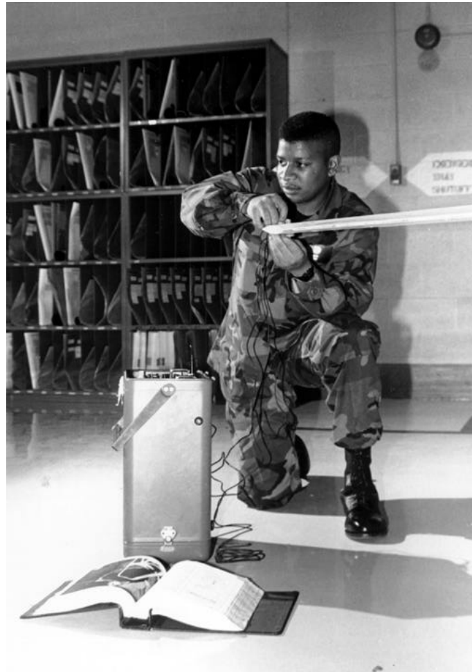
Figure 5-69. Typical Through-Transmission Inspection of a Stabilator.
