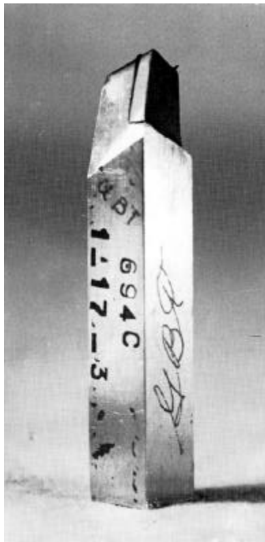
Figure 3-47. Magnetic Particle Indication of the Braze Line of a Brazed Tool Bit
